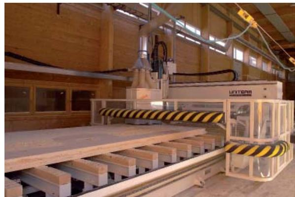
Figure 3: Manufacture of CLT (Courtesy of KLH)
